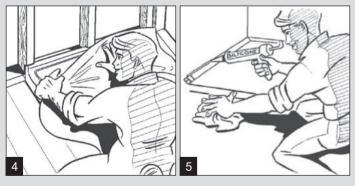
Water resistant plaster board installation. The SMC shower base has a 9mm tile flange. Place base against framework, install water resistant plaster board directly on top of tile flange and seal the joint with flexible silicone sealant.
