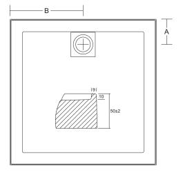
The self-supporting polymarble Daintree shower base features a square dome outlet and has a standard 9mm tile flange on all sides.
